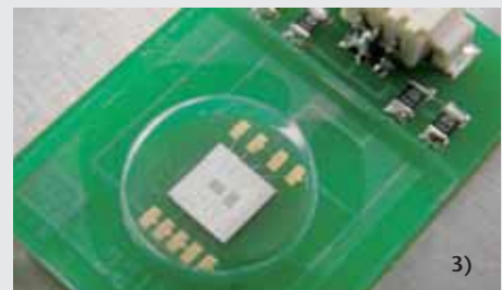
In-plane motion (1) and vibration spectrum (Bode plot) (2) of a MEMS comb drive (3)
