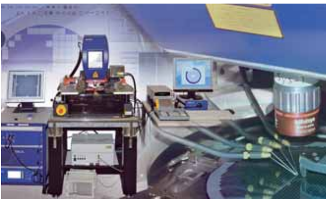
Semi-automatic probe station for production testing of pressure sensors (Melexis)
