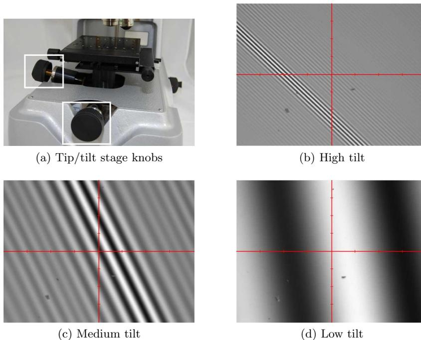
Figure 2.6: Tip/tilt Control &amp; Tilted Fringes
