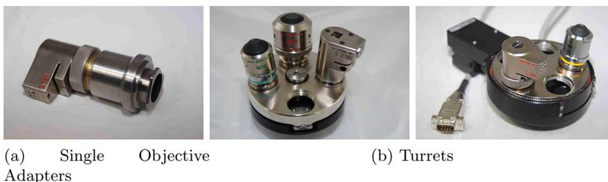
Figure 2.8: Objective Mounting Methods
