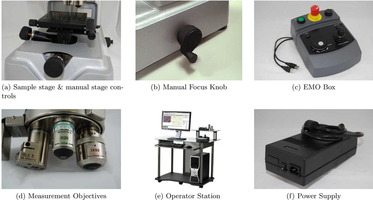
Figure 1.3: System Components
