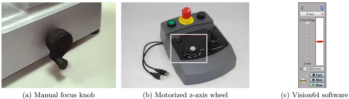
Figure 2.4: Focus Adjustment Mechanisms
