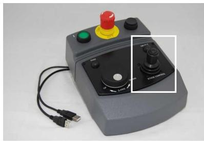
(b) Joystick for X/Y adjustment
